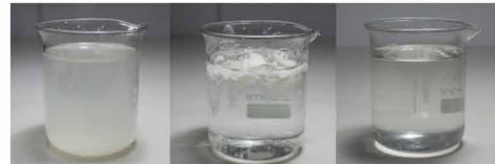
Surface treated type: Delayed solution None-surface treated type: Fast solution and get lump Liquid after solution
